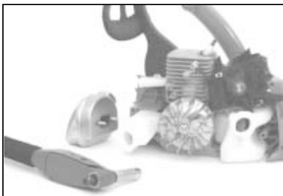
10-01 Removing the driving mechanism Only remove ignition and flywheel if cylinder is to be replaced.
