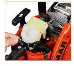
Installation and removal of the air filter requires no tools
